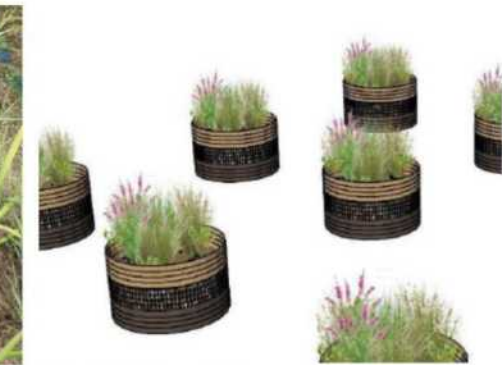
Intertidal tiered Ecosystems: steel gabions filled with estuarine sediment
