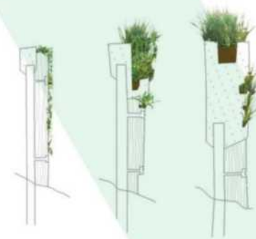
Timber cladding attached to vertical seawall. Gap backfilled with rubble and sediment to form vertical beach habitat and planted with intertidal plants
