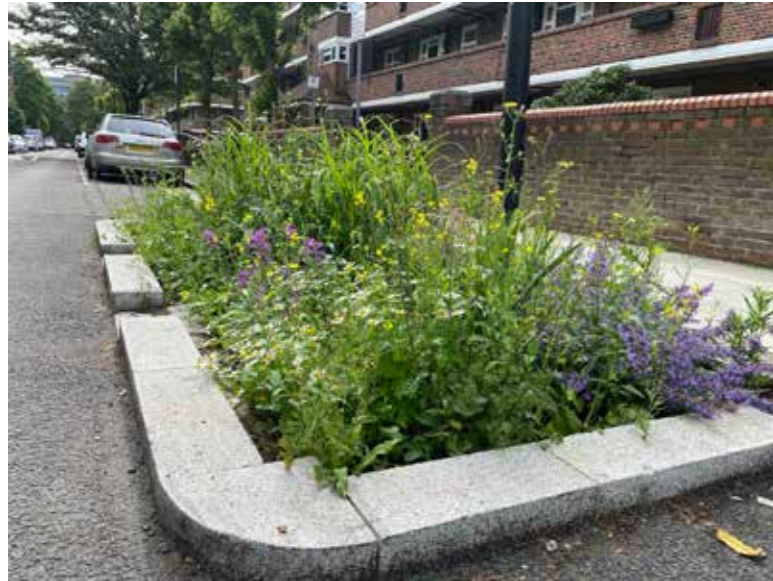
Reduce on-street parking by introducing kerb side rain gardens that collect rain water and bring it into the greenspace.
