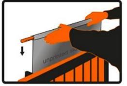
Position Radklips on wall brackets. If needed, roll more or trim bottom.
