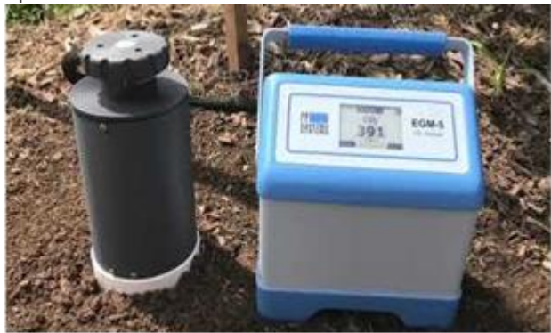
Figure 4. EGM machine (right) pictured with soil respiration chamber (left) used to measure the rates of respiration of soil microbes.
