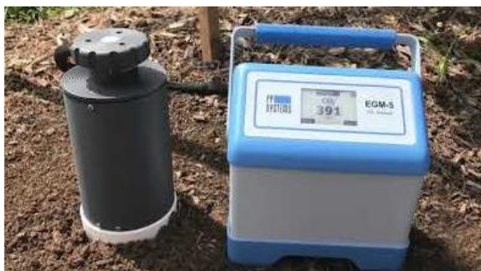
Figure 4. EGM machine (right) pictured with soil respiration chamber (left) used to measure the rates of respiration of soil microbes.
