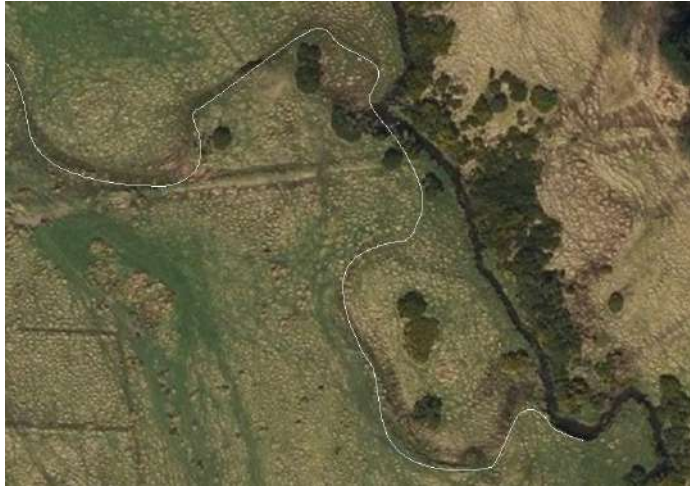
Paleochannels can be identified most easily using images from a drone. Here, the former pathway has been underlined to make it easier to see.
