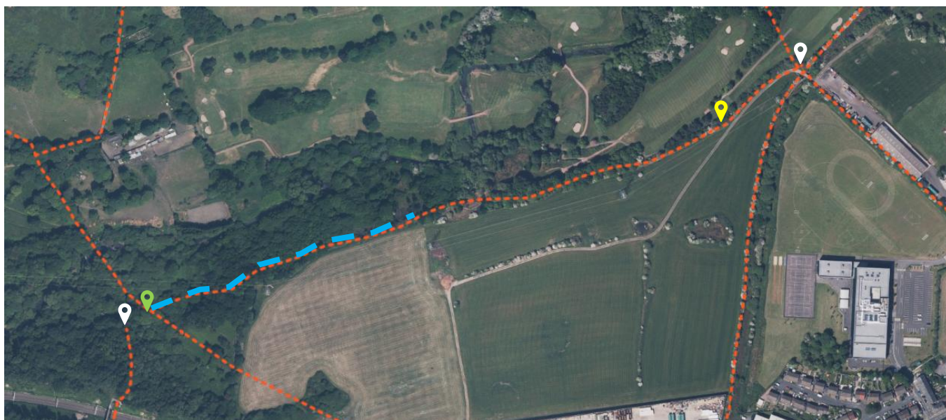
Fig 18: Proposed location of fingerposts (white), bridge (green), replaced stile (yellow), step renovation (blue)
