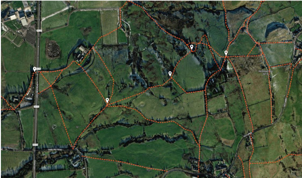
Fig 10: Proposed fingerpost locations (white), location for kissing gate installation and stile removal/replacement
